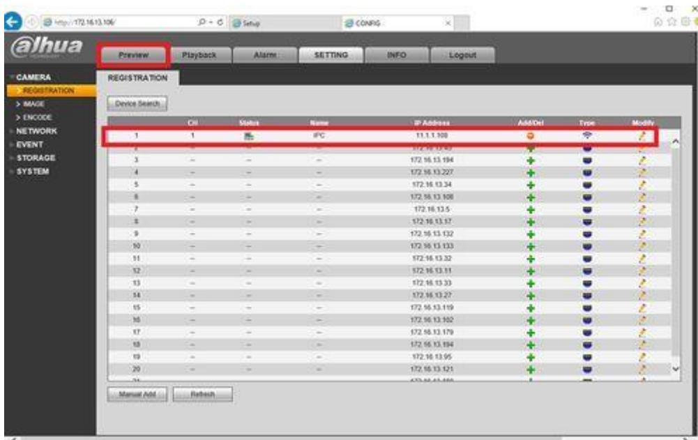
10. Select Preview and then the Camera that was added to ensure the stream is running correctly. At this time you can disconnect the wireless camera from the wired network and install it where there is wireless coverage.
